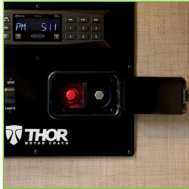
Garage Jumpstart Charging Center
