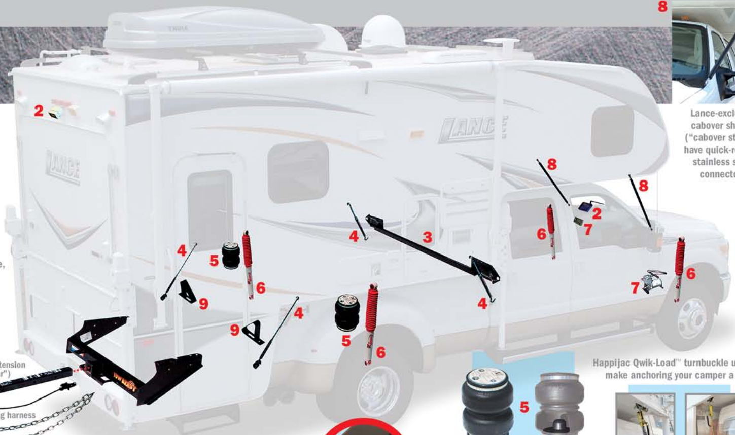
Within Air Lift's Super Duty air springs ("air bags") are the Lance-exclusive internal jounce bumpers
