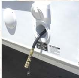
Exterior propane connectors
