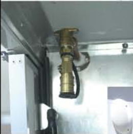
Exterior propane connectors
