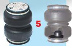
Within Air Lift's Super Duty air springs ("air bags") are the Lance-exclusive internal jounce bumpers
