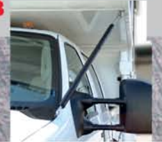
Lance-exclusive cabover shocks ("cabover struts") have quick-release stainless steel connectors
