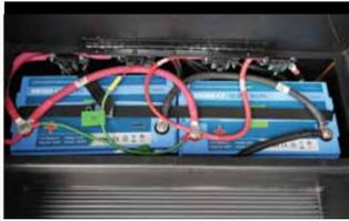
**Dual Low-Temp Lithium Auxiliary Batteries (200Ah Total)**
