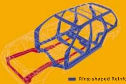
Ring-Shaped Reinforcement Frames in the front, center and rear of the Outback work with reinforced side sills to disperse the energy of an impact around the passenger compartment, offering added protection for occupants. Interior trim surrounding the windows and pillar areas is specially designed to absorb occupant impact during a collision to help reduce injury.
