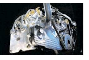
Outback is powered by a 2.5-liter, 16-valve horizontally opposed boxer engine producing 165 horsepower and 166 lb.-ft. of torque for low-end power. The engine's lower center of gravity design means reduced body roll in turns for secure handling.
