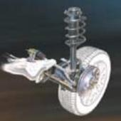
The 4-wheel, fully independent suspension has been designed to be extremely strong, yet supple and responsive on the road. In front, MacPherson struts use L-shaped lower arms for added rigidity and durability. Liquid-filled suspension bushings absorb unwanted vibration.
