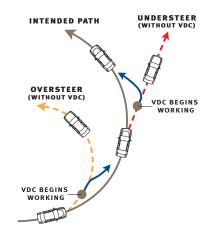
Subaru VDC helps the driver maintain directional control under all driving conditions. Using inputs from the steering angle, yaw rate, lateral g-force and other sensors, the VDC system monitors vehicle stability
