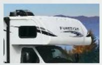
Seamless front cap for enhanced aerodynamics
