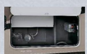
**HEATED AND ENCLOSED HOLDING TANKS**
