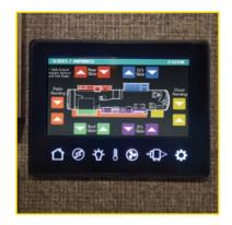
Multiplex Wiring Control System with 7" Touchscreen
