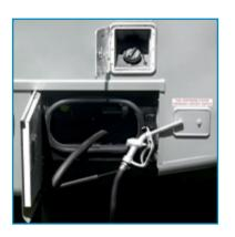
Remote Fuel Filling Station with Auxiliary Fuel Tank,
