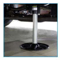
Automatic Leveling Jacks with Touch Pad Controls
