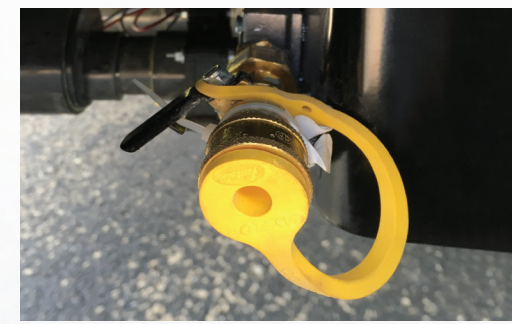
LP Quick Connect Each Isata 3 comes with an LP quick connect for use with a portable grill.
